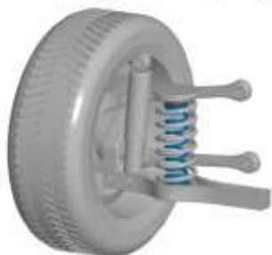
Auxiliary Coil Springs HV-.....5 mounted in original main spring
